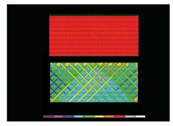
Figure 3. Stress distribution in the model representing diagonal type fibre design (Ribbond Triaxial). The colour scale indicates that stress is reduced throughout the model when compared to Figure 2. Diagonal fibres appear to absorb stress (yellow; 1.1-1.32 MPa).
