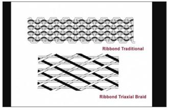
Figure 1. Schematic representation of Ribbond Traditional and Ribbond Triaxial.
