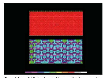
Figure 4. Stress distribution in a model representing leno weave-type fibre design with a lock-stitch feature (Ribbond Traditional). The stress values which were obtained in Figure 2 and 3 are reduced by 30% in this model (From 1.3MPa to 0.8 MPa). The high stress areas (green) are reduced and low stress areas (blue & violet) are increased when compared to the previous two models.
