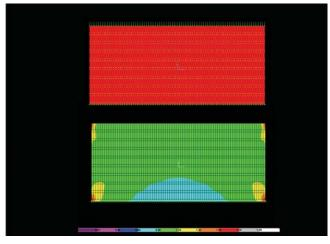
Figure 2. Stress distribution in the model representing unidirectional fibre design. All nodes at the bottom border of the model have been constrained. Load has been applied to all the nodes at top border of the model. An increased stress is observed in the corners (red-yellow;1.1-1.75 MPa). A homogenous stress distribution is observed all around the model (green; 0.88-1.1 MPa). This stress is reduced at the bottom of the model (blue; 0.66-0.88 MPa).
