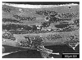
Figure 5. SEM image of composite resin reinforced with polyethylene fibre. fibre and horizontal crack in resin stopping at fibre (arrows) (With permission of Brendan F. Grufferty) <sup>66</sup>.
